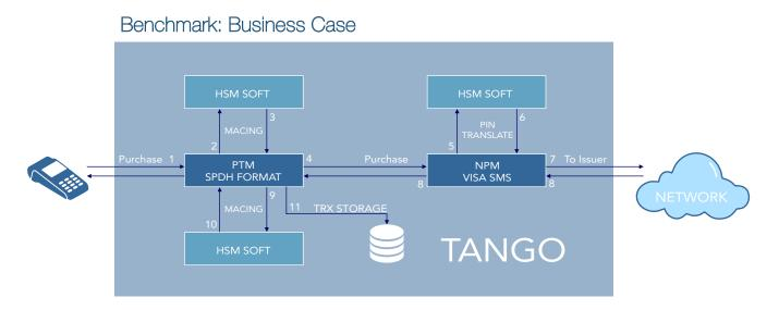
In this business case scenario we first simulate POS purchase transaction in TANGO. The message is then reformatted and sent out to the VISA simulator for authorization. On the reply we reformat the message to send to the POS device followed by a log to the database.
