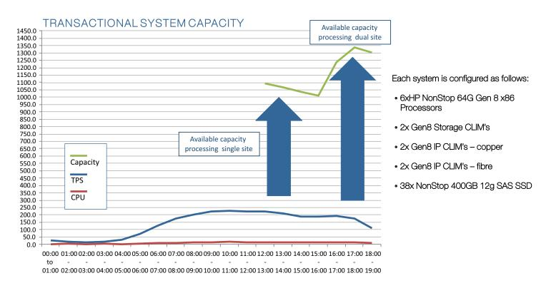
Bankserv Africa's Production and Test systems feature the same configurations therefore enabling like for like testing capability with regards to hardware, software and fail over scenarios. Their target was set at 600 tps. With the NonStop X, SSD and configuration, Bankserv Africa was able to see their systems have the capacity to achieve up to 1400tps, which over sought their target tremendously.
